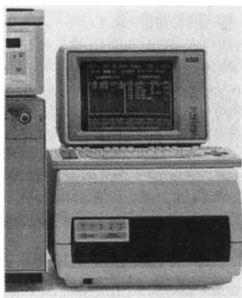
FIGURE 83. Varian 9060 DAD showing the optical unit/processor (bottom) and video screen/keyboard (top). (With permission.)
