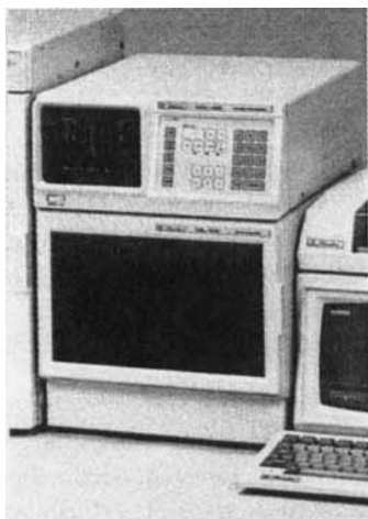
FIGURE 15. Shimadzu SIL-6A autosampler (bottom) and SCL-6A System Controller with video screen (top). (With permission.)
