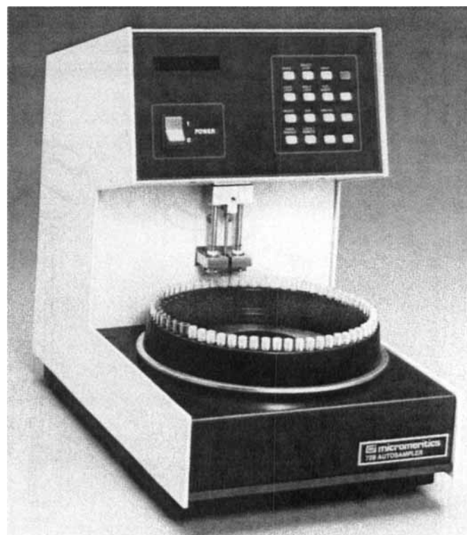
FIGURE 4. The Micromeritics 728 autosampler. The older 725 looked and operated similarly, but the 728 is more versatile. (With permission.)
