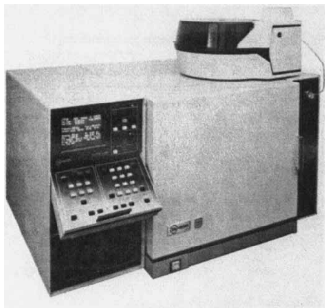
FIGURE 48. Varian 5000 rapid-refill, one-piston pump and low-pressure three-eluant gradient controller. (With permission.)
