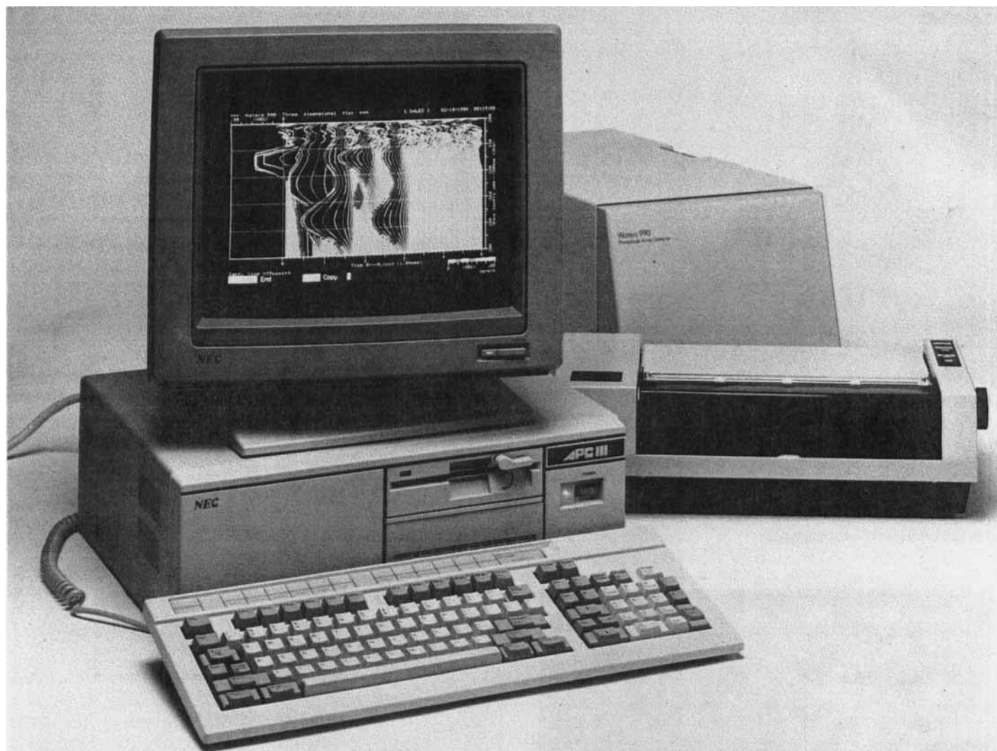
FIGURE 76. Waters 990 DAD showing the computer (left) and optical unit (right rear), and printer (right front): The three-dimensional perspective plot on the color screens shows wavelength (top to bottom), elution time (left to right), and absorbance (the visual vertical rise of the absorbance). The view can be rotated around the vertical (absorbance) axis and tilted on the wavelength-time plane.
