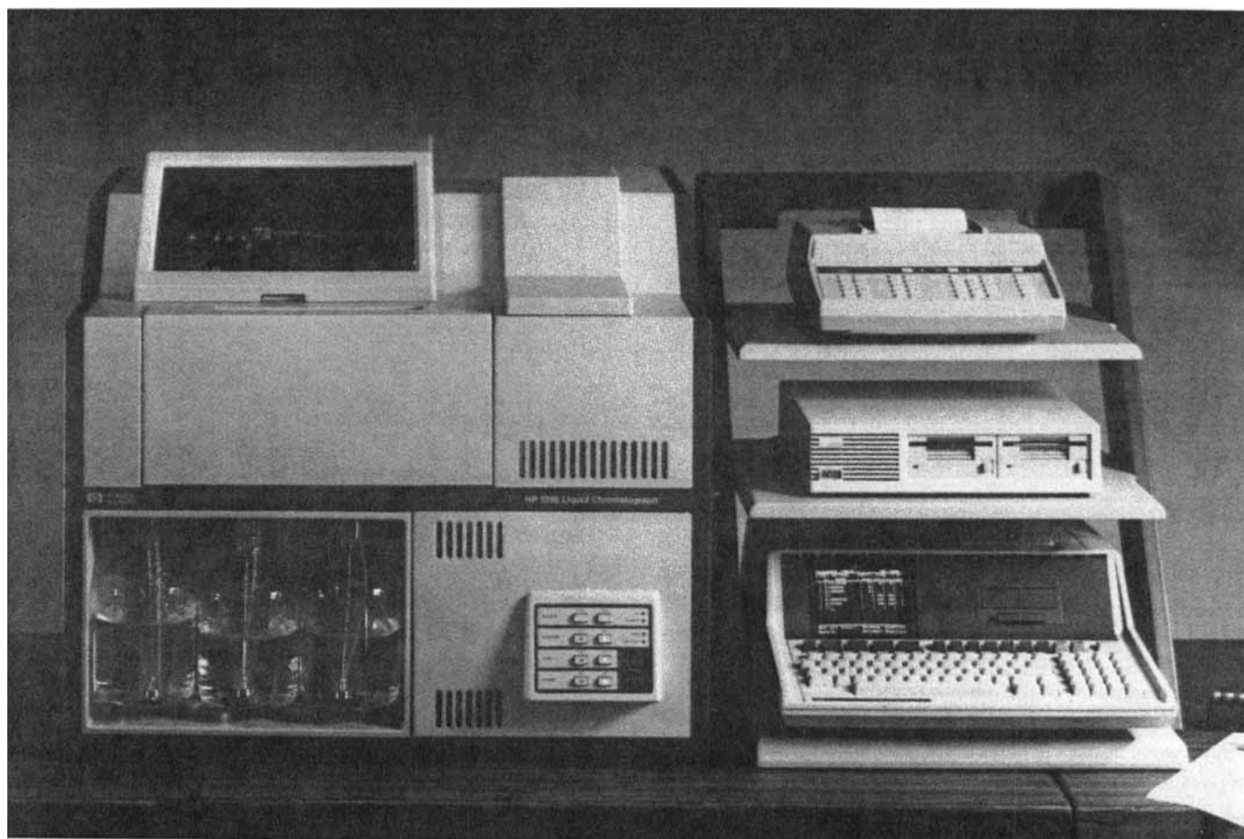
FIGURE 13. The Hewlett-Packard 1090 liquid chromatograph (left); the HP-85 PC (right, bottom); HP9121D disk drive (right, middle); and HP3392A Integrator (right, top). (With permission.)
