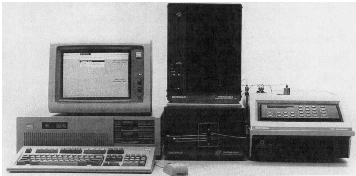
FIGURE 69. Beckman-Altex System-Gold "Amino Acid System", showing a 506 autosampler (right), 135 column Heater and 231 Post-Column Reactor (not shown), a 126 two-eluant pump module (with two rapid-refill one-piston pumps) (center) on top of a 116 Programmable visible detector, next to an IBM PS/2 Model 50 PC (left). (With permission.)
