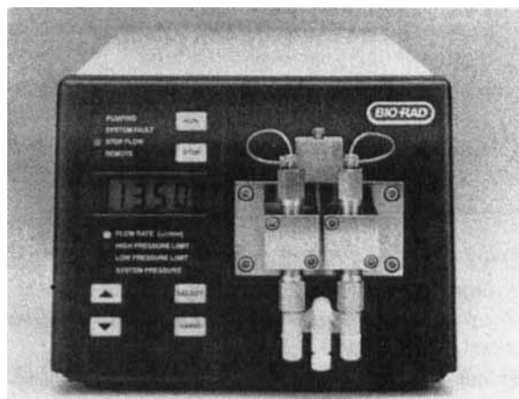
FIGURE 66. Bio-Rad 1350 "soft-start" parallel flow two-piston pump with electronic flow feedback. (With permission.)
