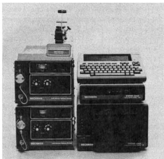
FIGURE 68. Beckman-Altex System-Gold "338 Gradient LC System", showing two 110B rapid-refill, one-piston pumps (left), controlled by a NEC lap-top computer (right, top), interfaced with a 406 Analog Interface Module (right, middle) and both sitting on a 116 Programmable UV/vis detector (right bottom). (With permission.)
