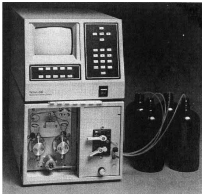
FIGURE 40. Waters-Millipore 600 parallel flow two-piston pump (bottom) with low-pressure three-eluant gradient controller (top). (With permission.)
