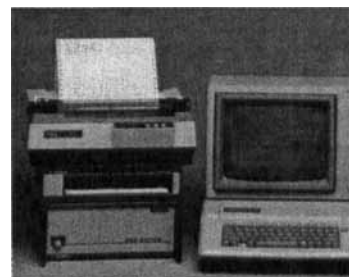
FIGURE 54. Gilson 704 high-pressure two-eluant personal computer (PC) based gradient controller and data system. (With permission.)
